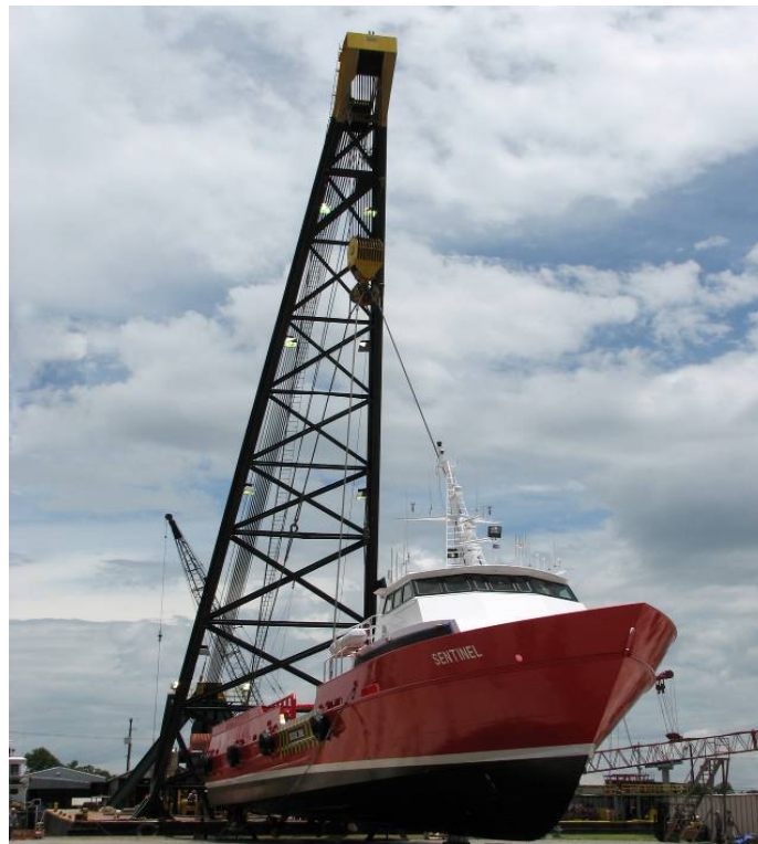
The D/B CAPPY BISSO launches a 200-ton crew boat in Harvey, La.
