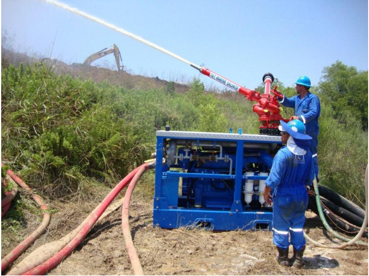
T&T Marine Salvage uses a 2,650-gpm fire pump system to help battle a landfill fire in Abbeville, La.
