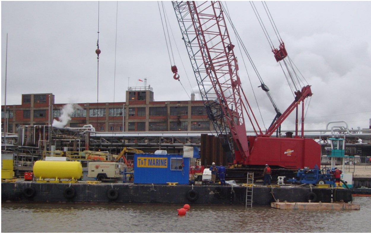
The C/B CURTIS T prepares a tugboat for lifting after it sank in the Houston Ship Channel.
